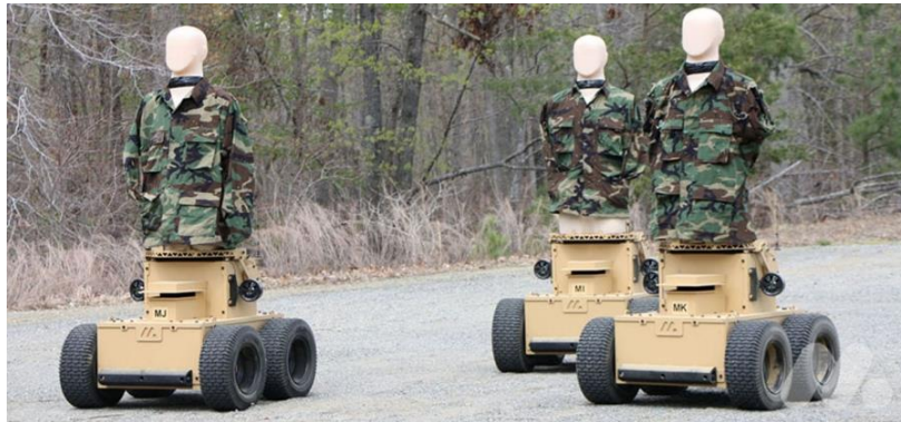
Figure 3: Robotic dummy with integrated fall-down mechanism upon “fatal” ballistic impacts
