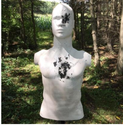
Figure 1: Rubber dummy with impact indication [2]
