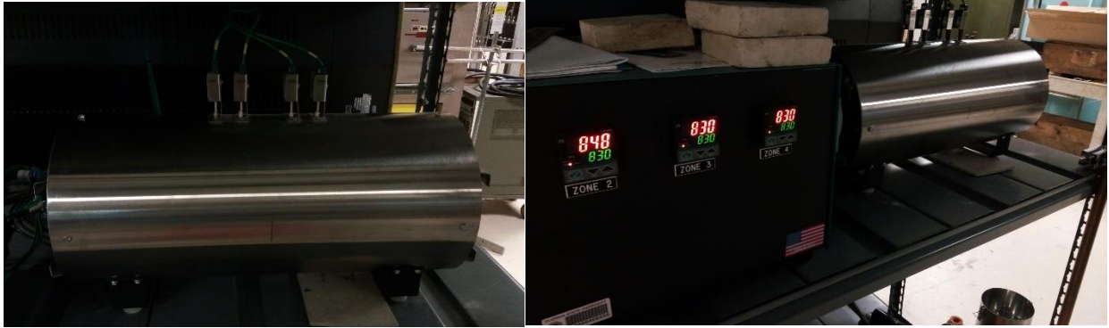
Figure 3: On the left is the furnace that was used and on the right is the power supply with the temperatures of each zone and the furnace.
