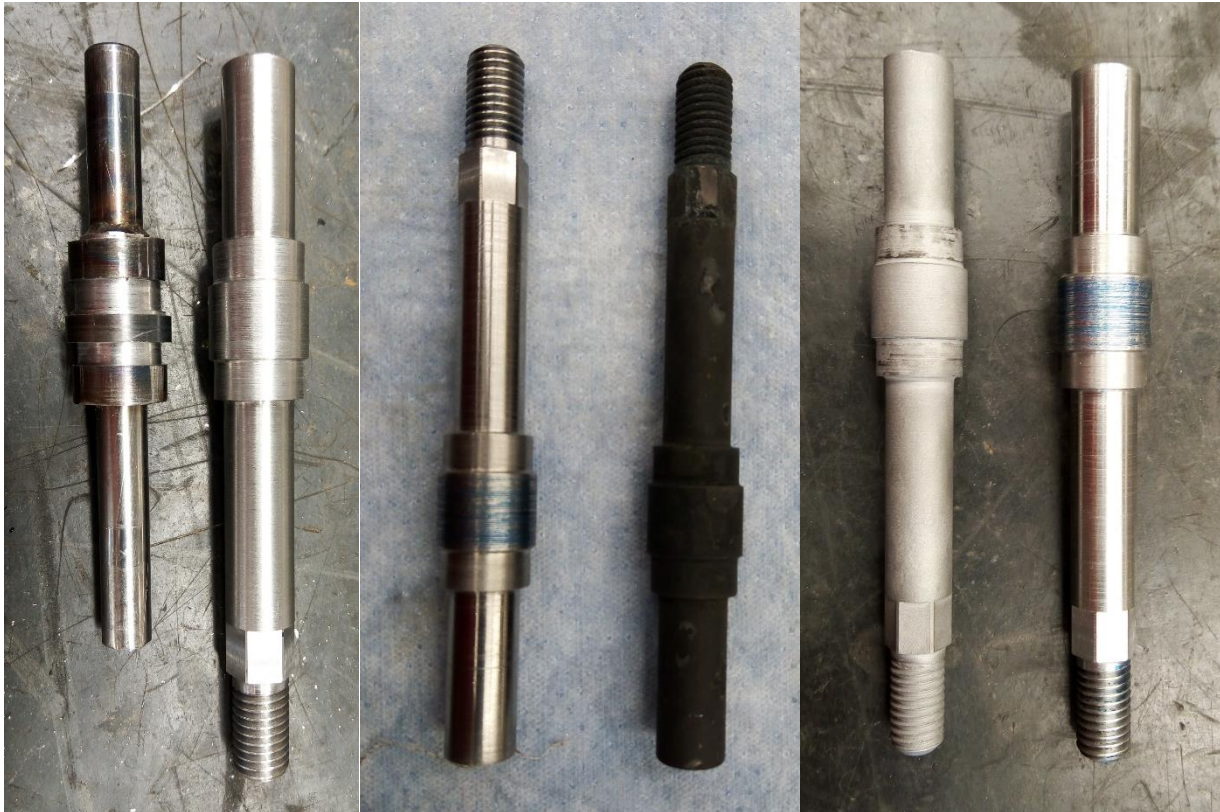
Figure 2: Original shaft vs new shaft (left), before and after heat treatment (middle), before and after the heat treated shaft was cleaned up (right).
