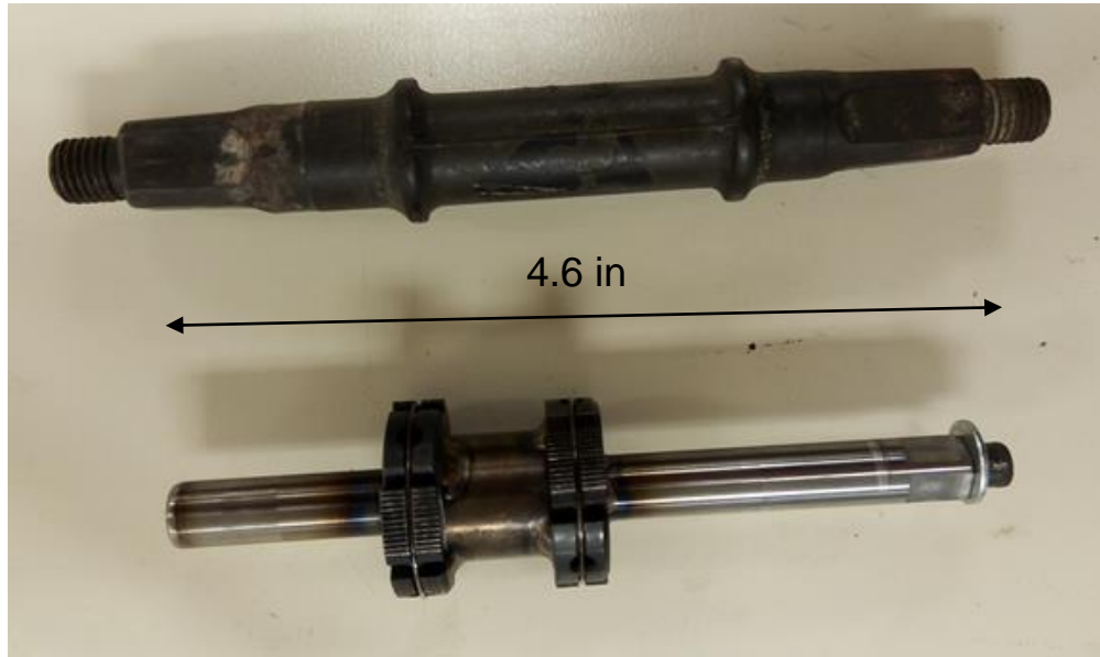
Figure 11: Traditional Bike output shaft (top) vs RLT Output Shaft (bottom)
