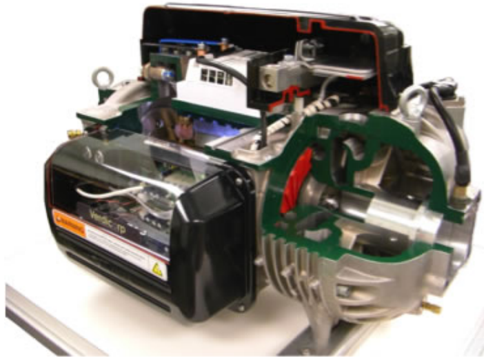
Figure 1. Verdicorp Cutaway Turbo Expander [1]
