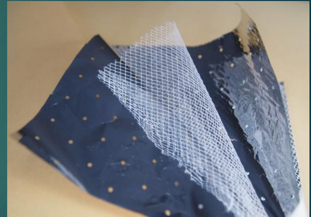
Figure 1 Layer of MLI with spacer
