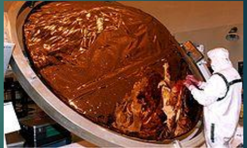
Figure 2 MLI being applied to a probe
