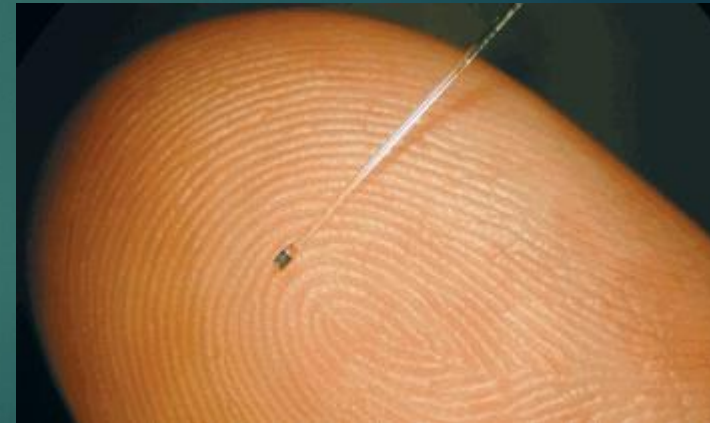
Figure 5 Fabry-Pérot Fiber optics pressure sensor size
