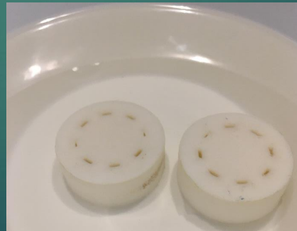
Figure 10 Mold dissolving in D-Limonene
