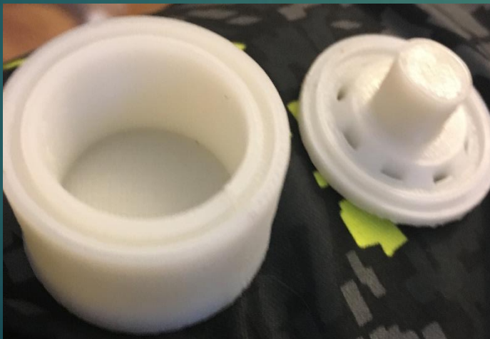
Figure 9 3D printed HIPS mold
