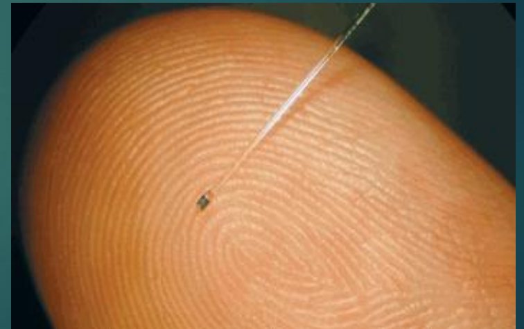
Figure 4: Displays the size of a fiber optics pressure sensor
