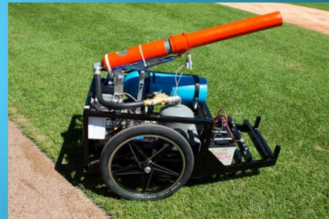
Figure 10: A larger air-powered cannon, the "Robo-Pitcher", is capable of 100MPH launch velocities [9]
