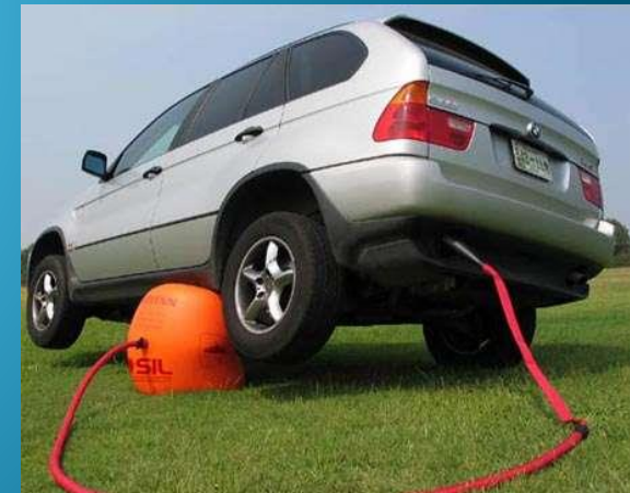
Figure 8: Inflatable jack in use [8]
