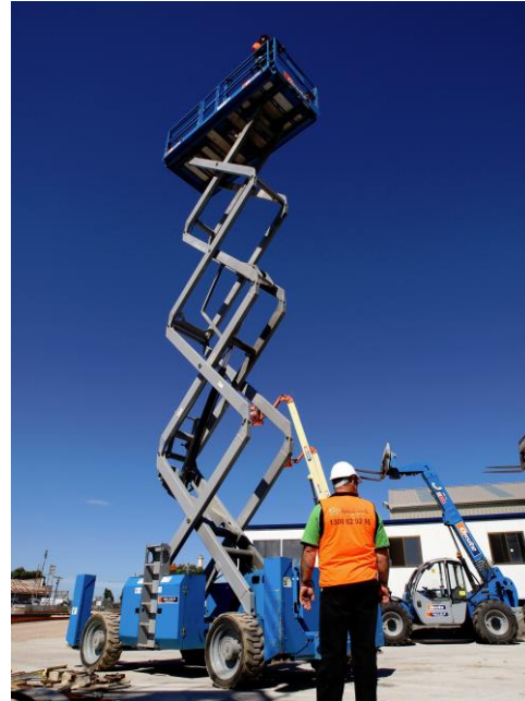
Figure 1b: A pneumatically-powered scissor lift using a vertically oriented input piston
