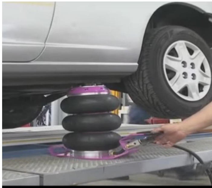
Figure 9: An example of an air jack in action. Team 23 is actively looking into using an air jack of similar construction to the one pictured.
