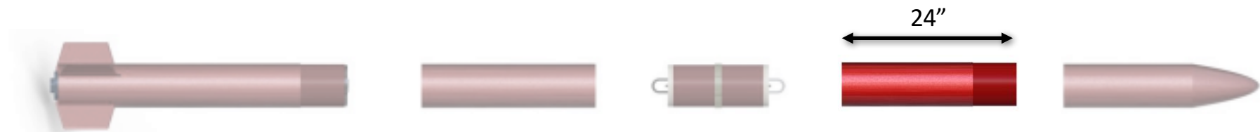
Figure 8: Main parachute bay
