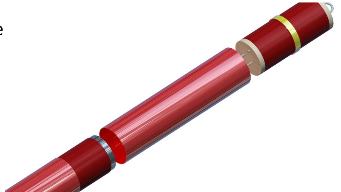
Figure 7: Separated drogue parachute bay.
