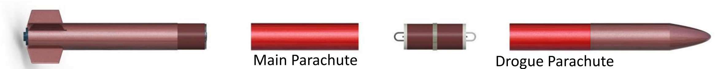
Figure 6: Separated drogue parachute bay.
