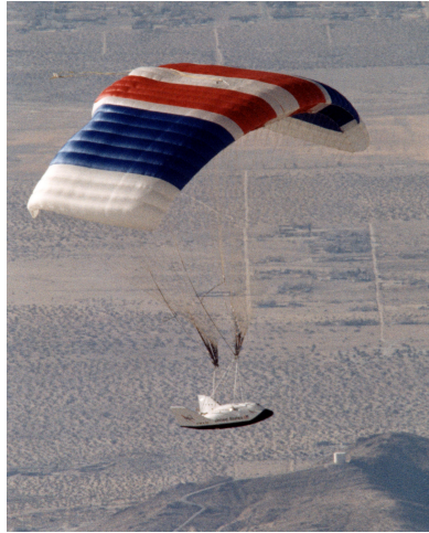
Figure 9: A steerable parafoil guiding an experimental flight vehicle. [8]
