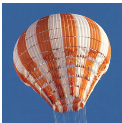
Figure 8: A large-scale reefed parachute system after deployment, still in its reefed stage. [9]
