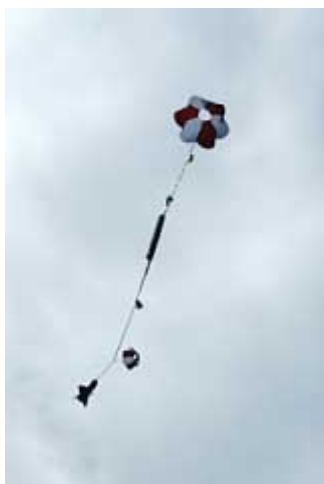
Figure 7: A dual deployment parachute system after deployment. [7]
