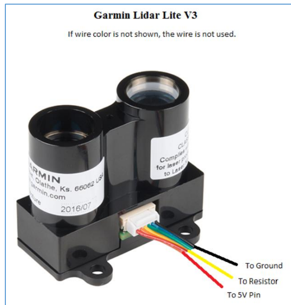
Figure A 10: LiDAR Lite V3 wiring
