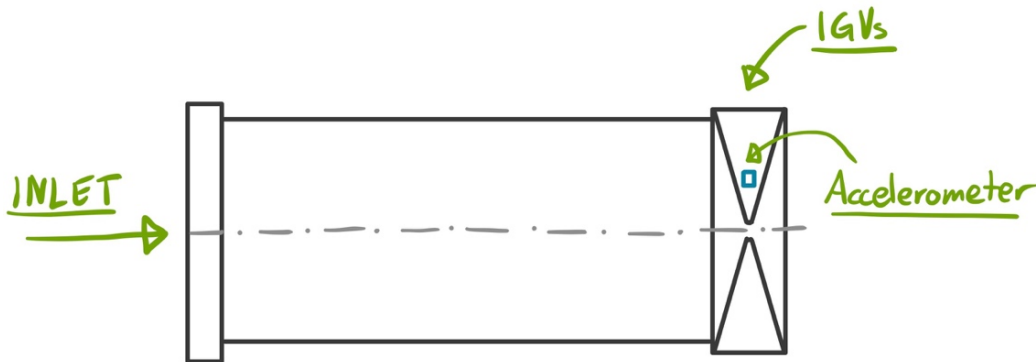
Figure 7. High cycle monitoring concept utilizing an accelerometer.
