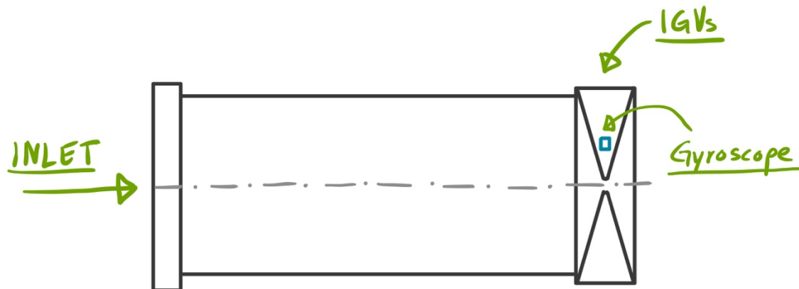
Figure 10. Angle monitoring concept utilizing a gyroscope.
