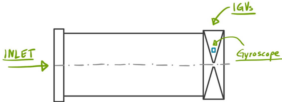
Figure 11. Angle monitoring concept utilizing a gyroscope.
