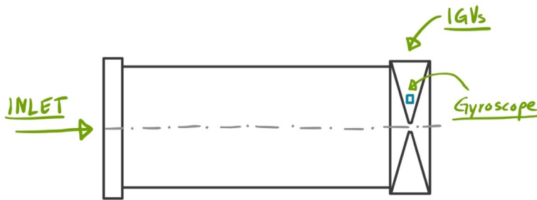
Figure 11. Angle monitoring concept utilizing a gyroscope.
