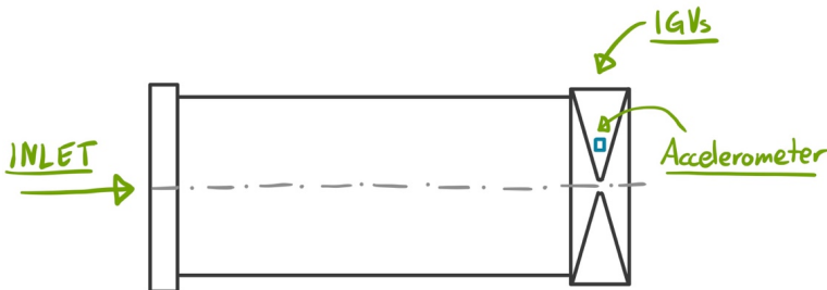
Figure 7. High cycle monitoring concept utilizing an accelerometer.
