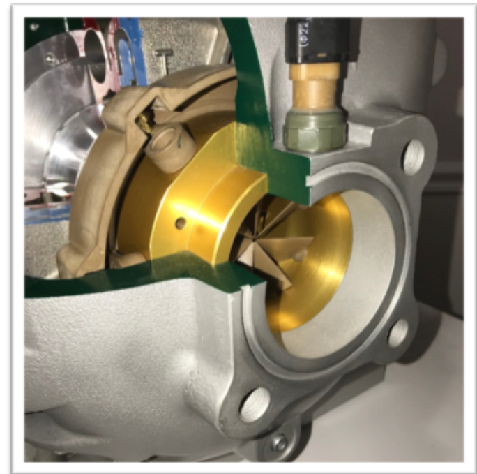
Compressor Inlet Cutout
