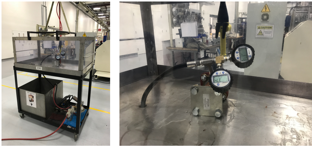
Figure 4. Pressure Burst Test Setup
