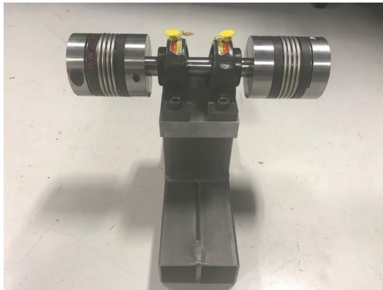
Figure 7: Mock Torque Transducer with BK2 Mock Shaft and BK2 Coupling Angle L's and Bolt Assembly
