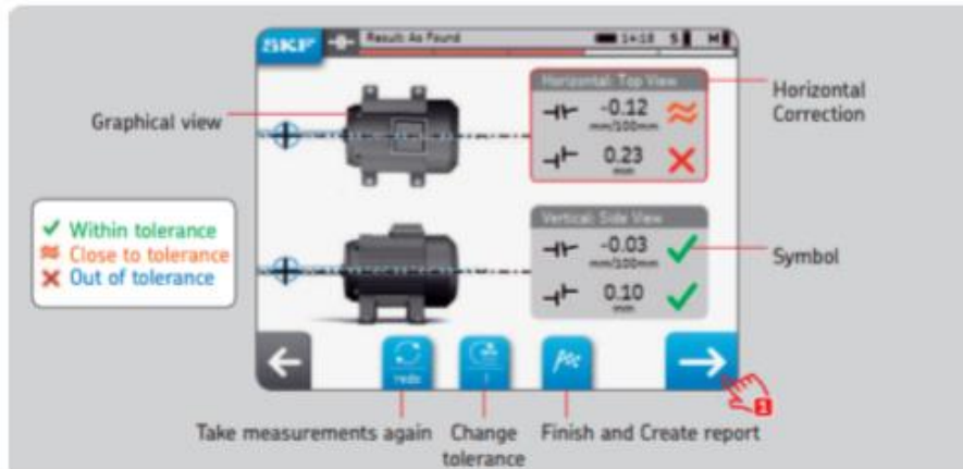
Figure 20: Horizontal Motor Alignment Live Feed
