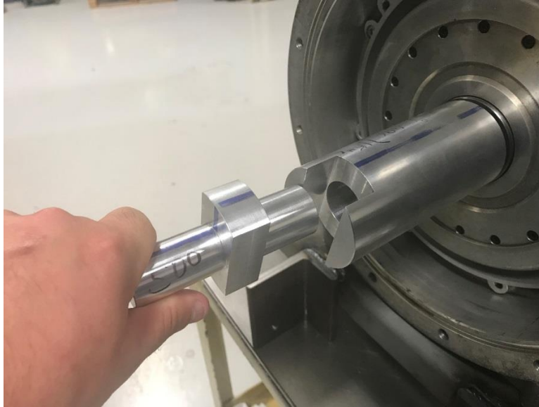
Figure 4: Connection of Coupler Connector to Shaft Extender
