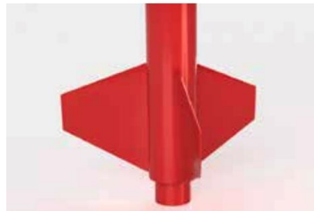
Figure 2.5.3 Tapered Fin Airfoil
