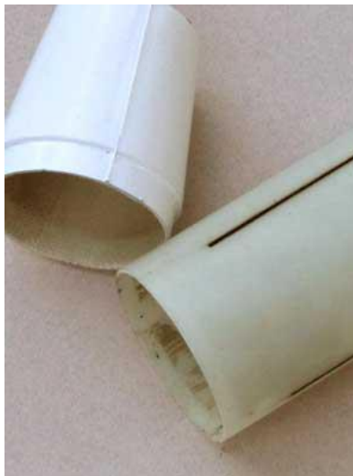
Figure 1.1.4 Fiberglass rocket body (right) with a cardboard nose cone (left).
