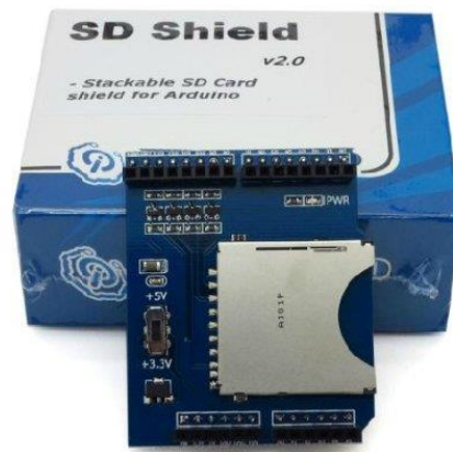
Figure (4.4.1) SD storage shield for Arduino
