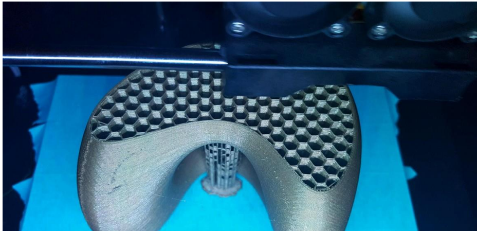
Figure 3.2.3.3 Natural honeycomb fill in a 3D printed piece.
