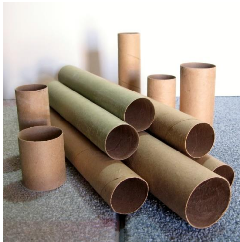
Figure 1.1.1 Multiple thin walled cardboard tubes to be used for rocket body.
