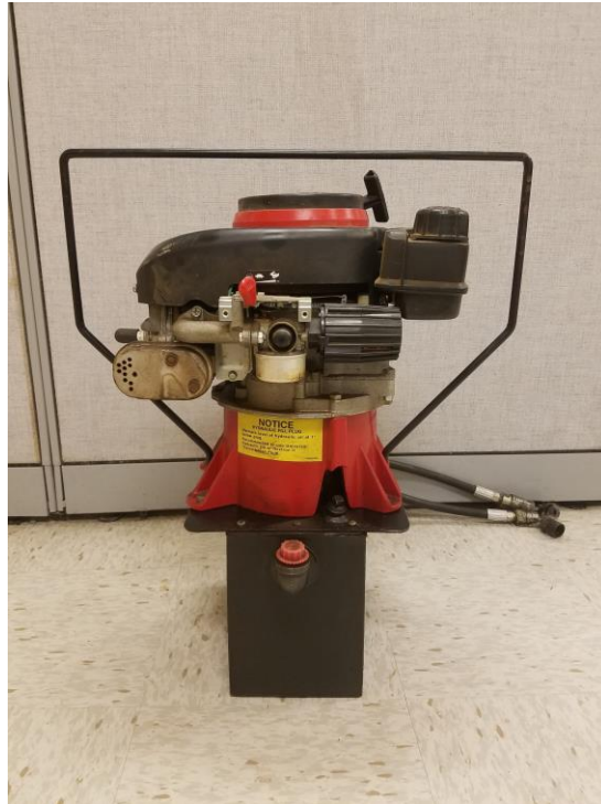
Figure 5: Reservoir, pump, and motor
