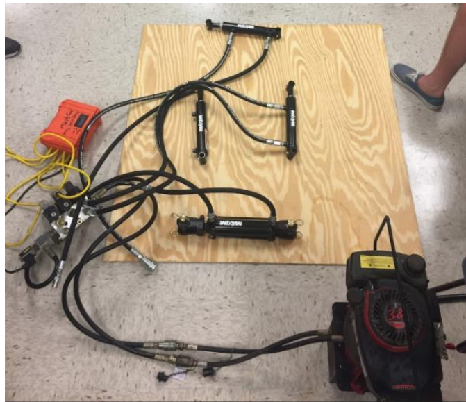
Figure 13: Assembly of hydraulic system
