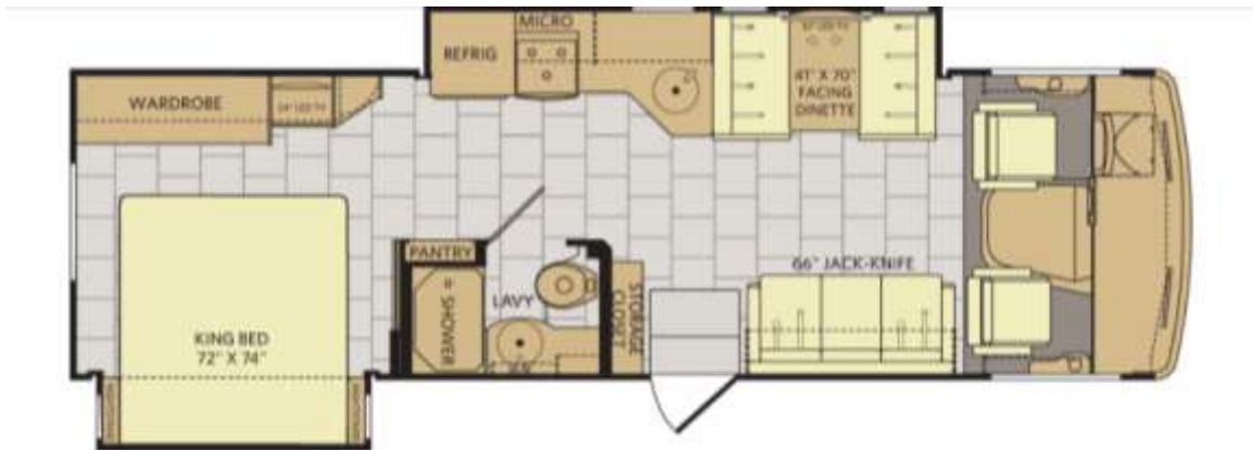
Figure 2. A basic layout of a motor home.
