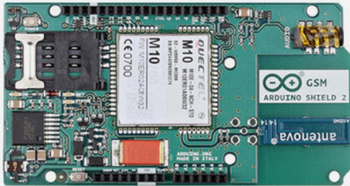
Figure 9. This figure shows the shield to use GSM capabilities with Arduino based microcontrollers (Arduino).
