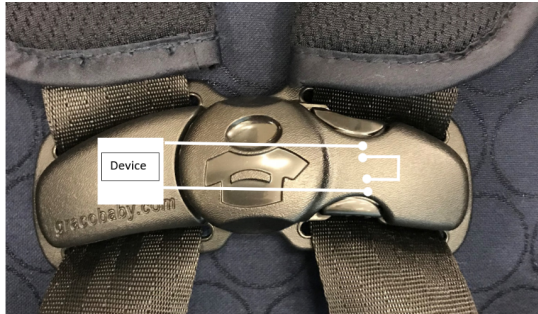
Figure 4: Device schematic to illustrate the closed circuit for activation of the device and verification that a child is in the seat (Graco Baby buckle used for illustration purposes).
