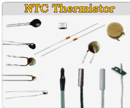
Figure 1. Image of different types of NTC thermistors (Arduino: Using NTC Thermistors).
