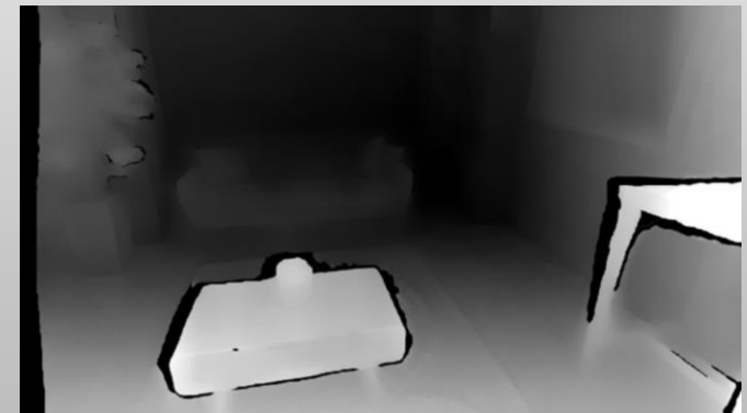
Fig. 12: ZED Stereoscopic camera maps distance in grayscale.
