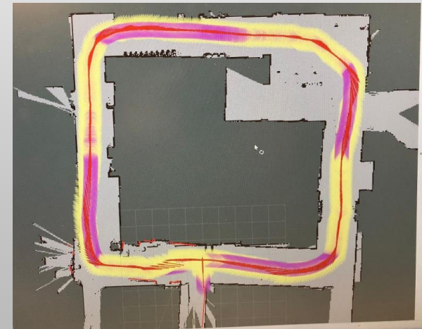
Fig. 20: Particle Filter Localization.
