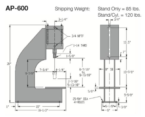
For non-standard double-acting service with strokes up to 6", use pages 30-31 to design a 6" bore cylinder for use with this stand.
