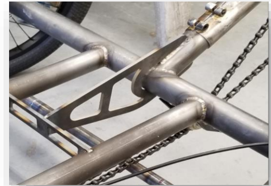
Chain Routing with brackets (Two redirection points)
