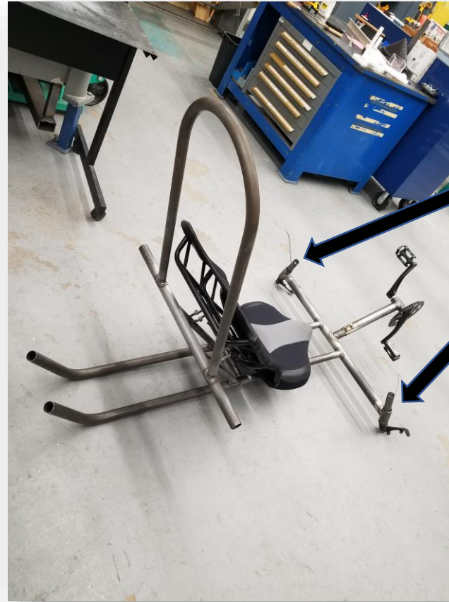
Prototype – January 14, 2019 Crossbar, Head tubes, Steering Knuckles, Pedals
