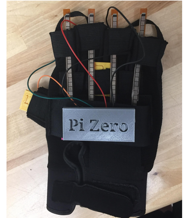
Figure 9: Flex Sensors, IMU's, Raspberry Pi Zero
