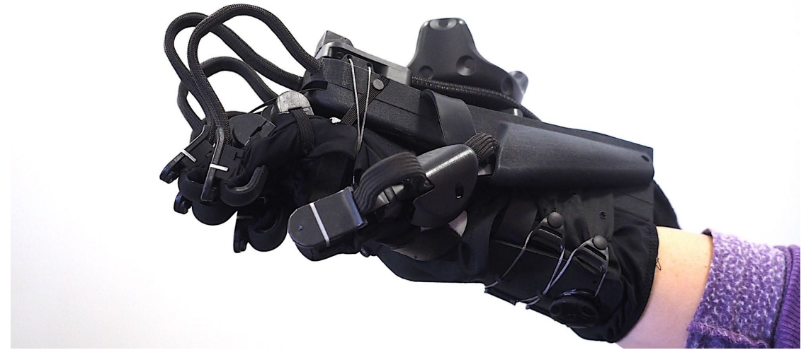
Figure 4: Example of current Haptic Feedback Glove (HaptX glove)
