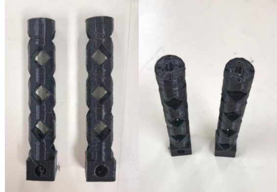
Figure 2. First iteration of 3D printed linkages.
