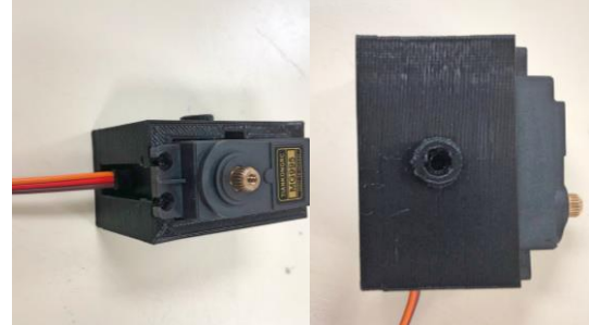
Figure 3. First iteration of 3D printed motor housing.
