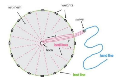
Figure 1. A diagram of a casting net commonly used for retrieving bait fish.
