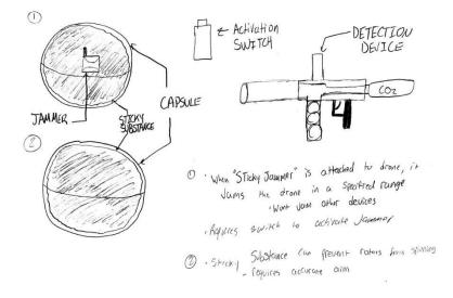
*Figure 1: Concept 1 diagram and detailed view of sticky substance*
