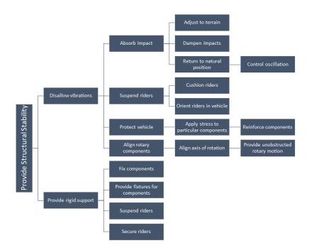
Figure 3.3.3 Provide Structural Stability Functional Decomposition Flowchart
