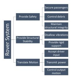
Figure 1.3.1 Device, System, Subsystem Functional Decomposition Flowchart
