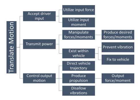
Figure 4.3.4 Translate Motion System Functional Decomposition Flowchart
