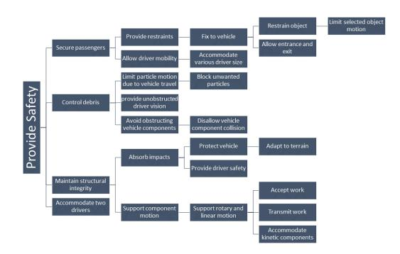
Figure 2.3.2 Provide safety System Functional Decomposition
