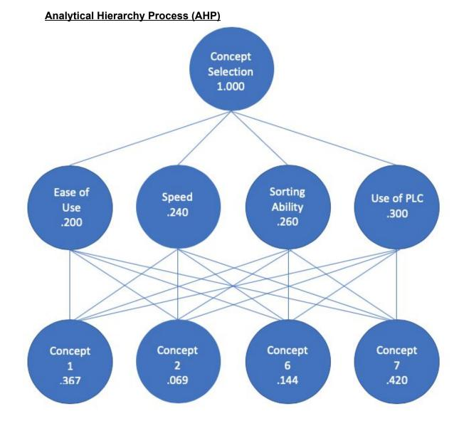
Using the top four criteria and concepts identified in the House of Quality and Pugh Charts, the Analytical Hierarchy Process chart was constructed above. Weighting the criteria respectively, the AHP chart awarded concept 7 with the highest score. Concept 7 was followed by concepts 1, 6, then 2.
