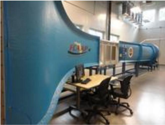
Figure 9: FCAAP subsonic wind tunnel
