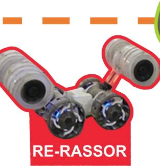
Due to the high cost of traveling to the moon, a NASA mining robot, RASSOR, could become a general-purpose robot. Astronauts could use RASSOR for different tasks by interchanging parts. This will reduce the amount machinery on the rocket, which in turn, decreases the cost. Our design is tested on the RE-RASSOR platform, a scaled down, fully 3D printed version of the original.
