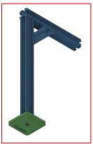
d. Lastly, using standard M8 bolts (S-M8) fasten the test assembly to the workstation through the test plate slots as shown below.
