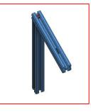
b. Fasten the gusset beam (L3) to the vertical (L1) and horizontal (L2) support beams using standard M8 bolts as shown below.
