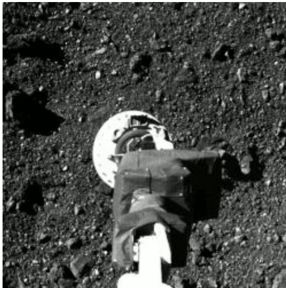
OSIRIS-Rex Using Nitrogen Blast to Collect Regolith
