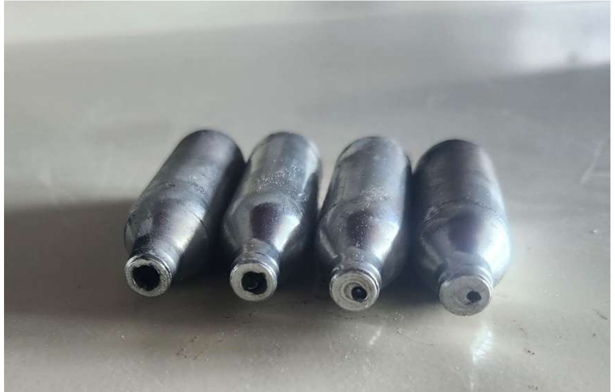
Tested 8g CO 2 Canisters Successful (Left); Malfunctioned (Right)
