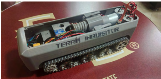
Figure 1: Final Terra Inquisitor layout showing FDM-enabled packaging of drive, drilling, soil collection, water delivery, and testing subsystems.
