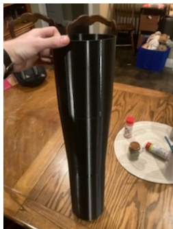
Figure 6: PETG printed mold used to form the custom 6-inch to 5-inch transition.
