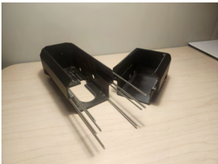
Figure 2: Split printed chassis reinforced with embedded steel rods for stiffness, printability, and sub-system integration.
