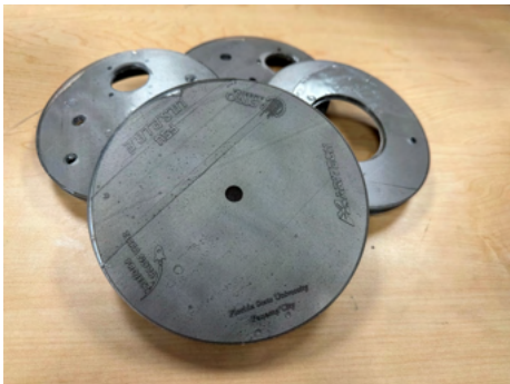
Figure 8: Laser powder bed fusion Inconel 718 recovery bulkheads used in the flight vehicle.
