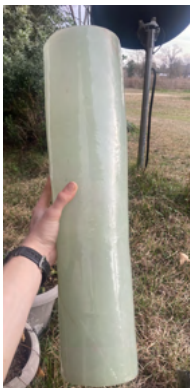
Figure 7: Fiberglass composite transition produced from printed tooling.
