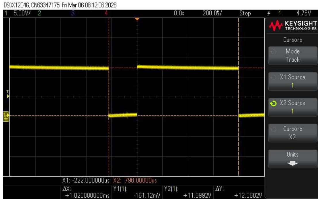
Figure 4.46 Unloaded Motor Driver Output
