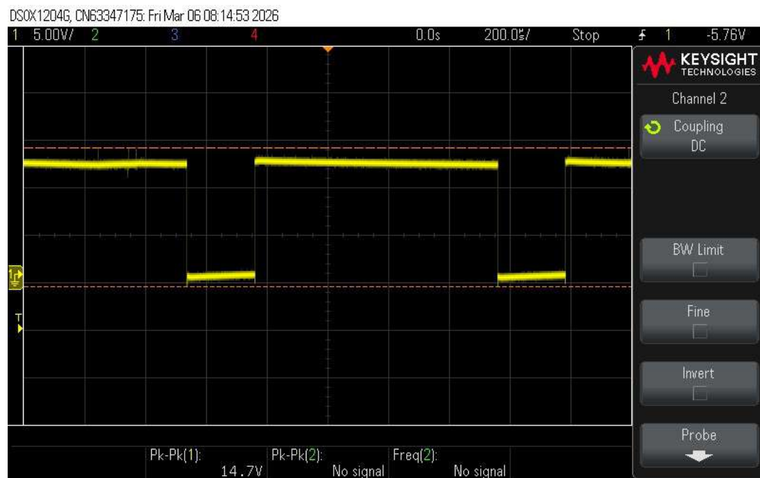
Figure 4.50 Loaded Motor Driver Output
