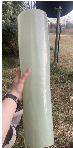
Figure 10: Transitional Airframe with Inner Mold Removed
