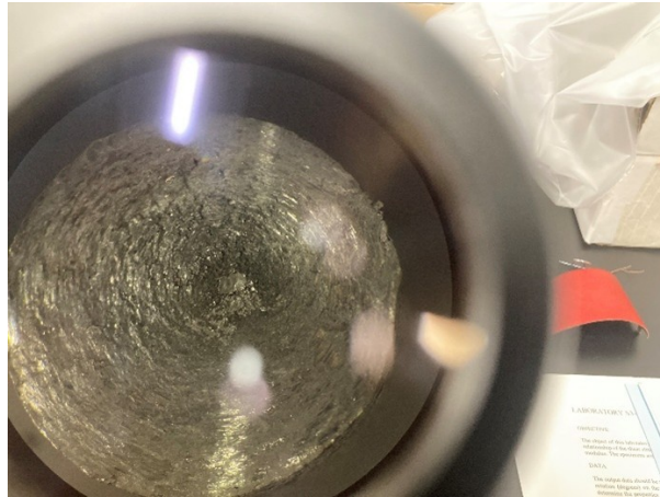
Figure 8: Fracture Surface of Heat-treated 3D Printed Inconel 718
