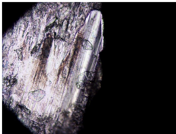
Figure 9: 20x Magnification of Heat-treated Inconel 718 Fracture Surface
