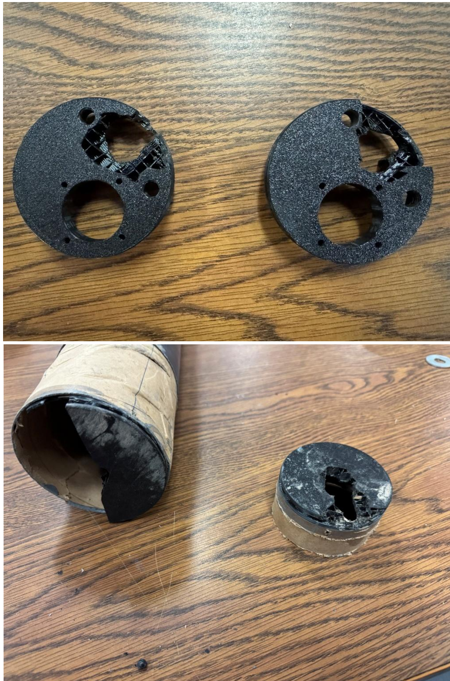
Figure 3-7 AV Bulkheads (Top), Fwd & Aft Bulkhead (Bottom)
