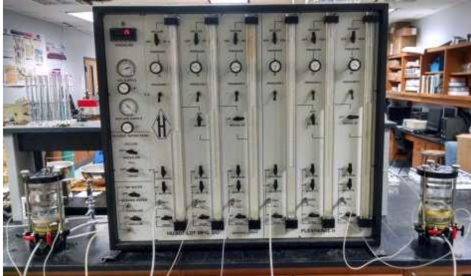
Figure 12: Flexible wall perimeter test setup to measure hydraulic conductivity
