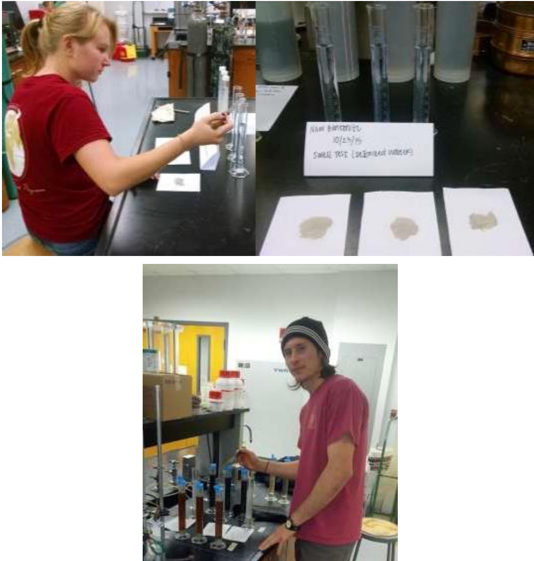
Figure 5: Swell Index Test conducted by Alyssa & Avery
