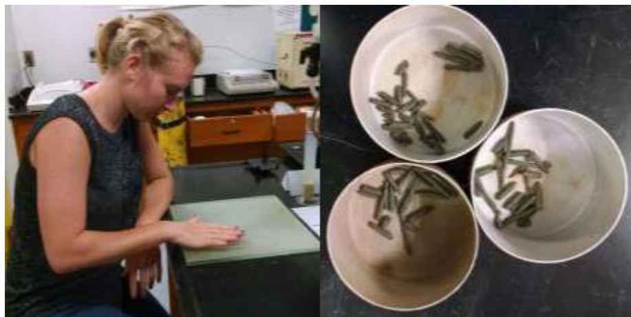
Figure 3: Plastic Limits Testing conducted by Alyssa
