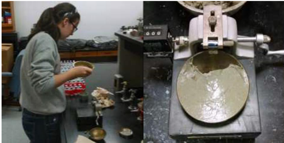
Figure 2: Liquid Limits Testing conducted by Nora & Tristan
