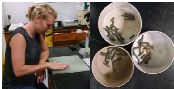
Figure 3: Plastic limits testing conducted by Alyssa
