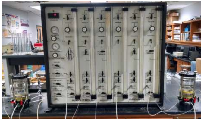
Figure 16: Flexible wall permeameter test setup to measure hydraulic conductivity
