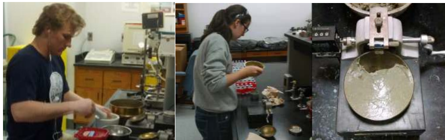
Figure 2: Liquid Limits Testing conducted by Nora & Tristan
