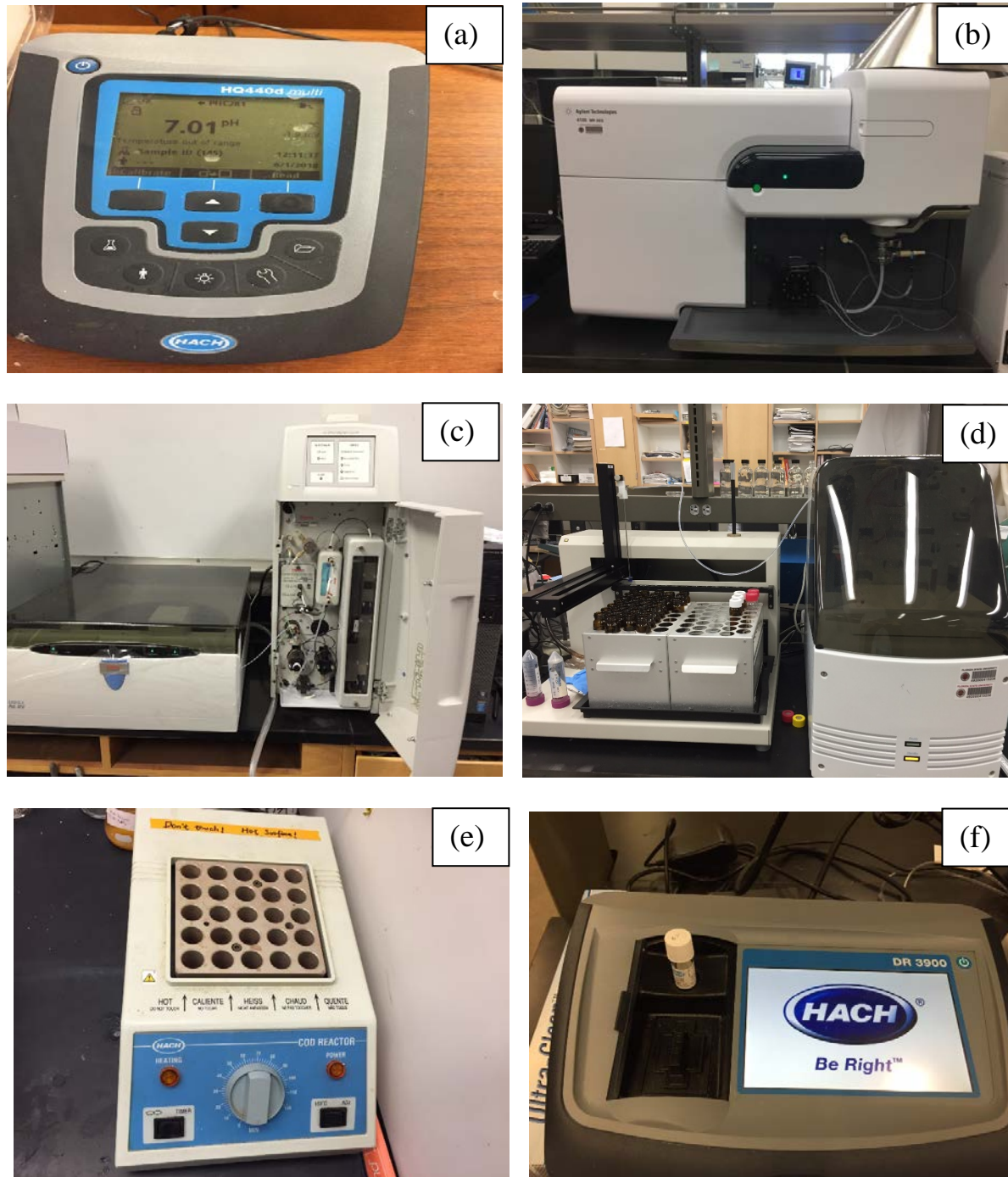
Figure 2. Instruments used for the leachate characterization: (a) Multi-parameter meter for pH, conductivity and ammonium measurement; (b) MP-AES for cation measurements; (c) IC for anion measurements; (d) TOC analyzer for TOC measurement; (e) COD reactor and (f) spectrophotometer for COD measurement.
