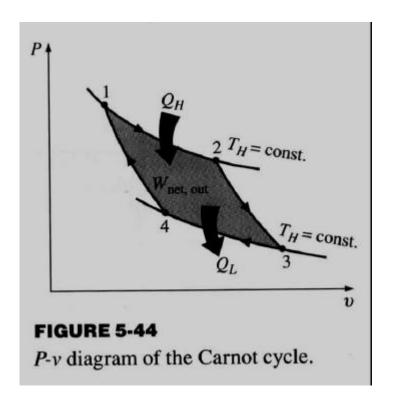
Work done by gas =  $\int PdV$ , area under the process curve 1-2-3.
