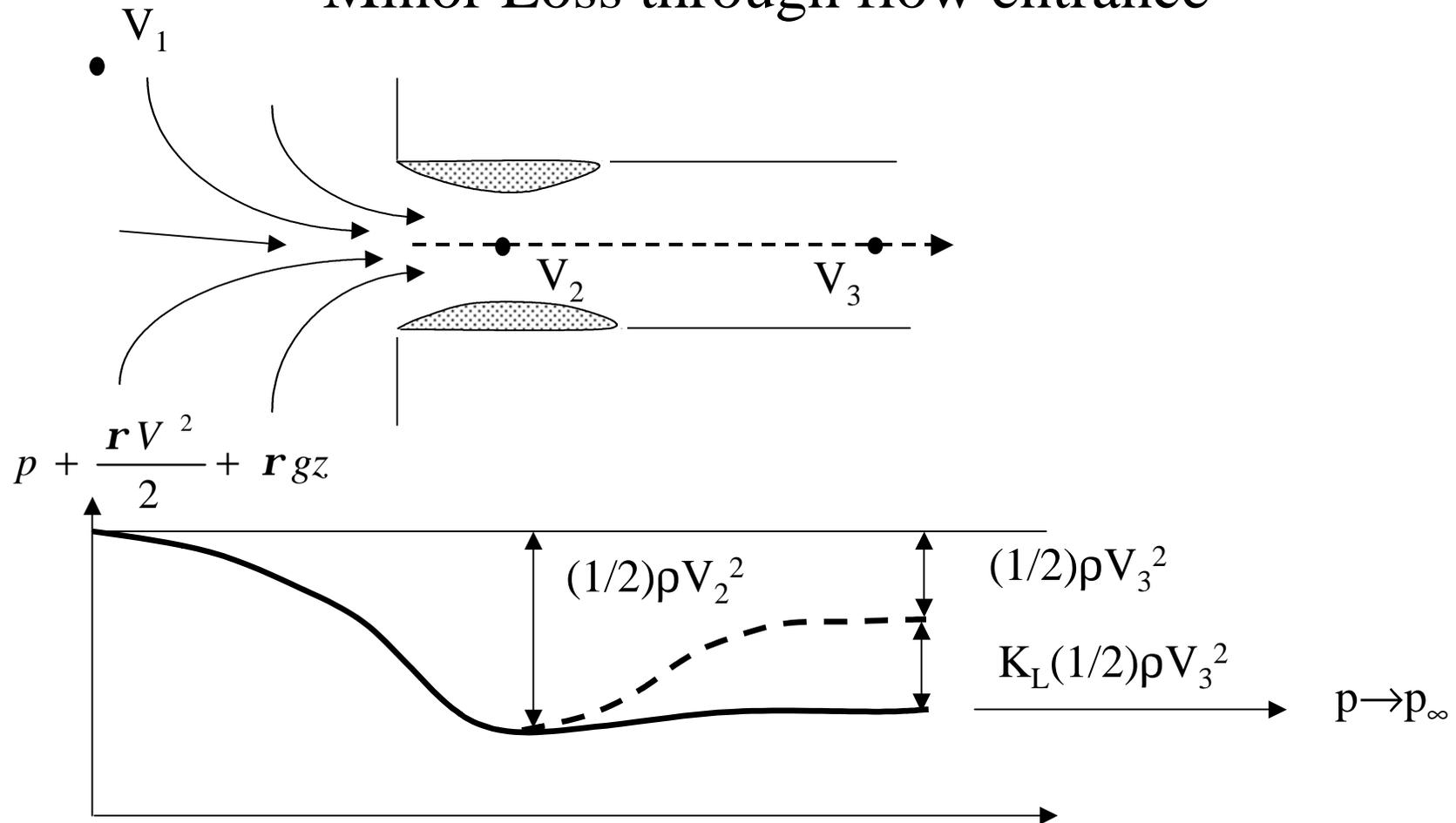
$$\text{Extended Bernoulli's Equation: } \frac{p_1}{\rho g} + \frac{V_1^2}{2g} + z_1 - h_L = \frac{p_3}{\rho g} + \frac{V_3^2}{2g} + z_3, h_L = K_L \frac{V_3^2}{2g}$$
