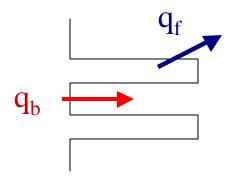
Define terms:  $A_b$ : base area exposed to coolant  $A_f$ : surface area of a single fin  $A_t$ : total area including base area and total finned surface,  $A_t=A_b+NA_f$  N: total number of fins
