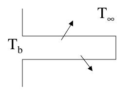
Total heat loss:  $q_f$ =Mtanh(mL) for an adiabatic fin, or  $q_f$ =Mtanh(mL<sub>C</sub>) if there is convective heat transfer at the tip
