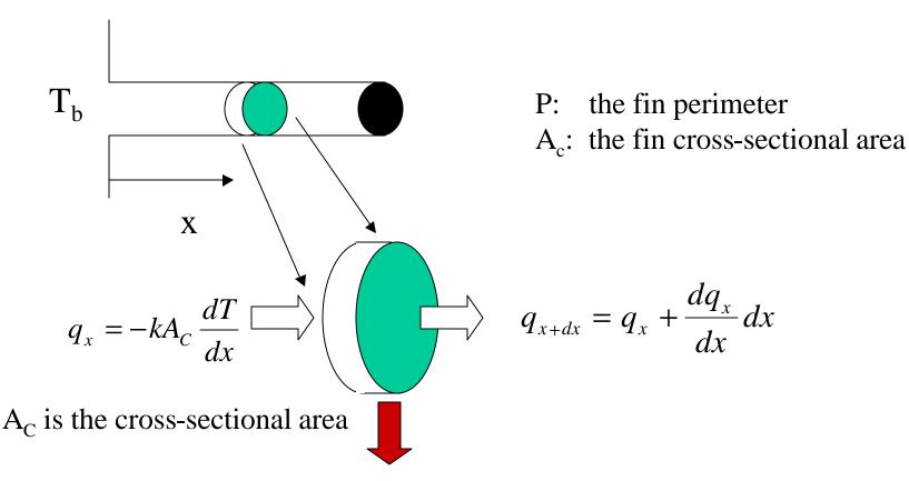
$dq_{conv} = h(dA_S)(T - T_{\infty})$ , where  $dA_S$  is the surface area of the element Energy Balance:  $q_x = q_{x+dx} + dq_{conv} = q_x + \frac{dq_x}{dx}dx + hdA_S(T - T_{\infty})$
