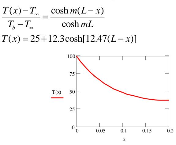
Temperature at the handle (x=0.2 m) is only 37.3 °C, not hot at all. This example illustrates the important role played by the thermal conductivity of the material in terms of conductive heat transfer.
