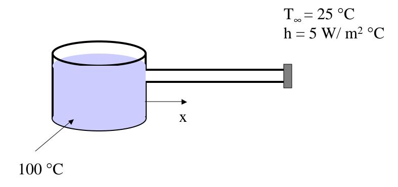
We can model the pot handle as an extended surface. Assume that there is no heat transfer at the free end of the handle. The condition matches that specified in the fins Table, case B. h=5 W/ m<sup>2</sup> °C, P=2W+2t=2(0.03+0.005)=0.07(m), k=237 W/m °C, A<sub>C</sub>=Wt=0.00015(m<sup>2</sup>), L=0.2(m) Therefore,  $m=(hP/kA_C)^{1/2}=3.138$ ,  $M=\sqrt{(hPkA_C)(T_b-T_{\infty})}=0.111\theta_b=0.111(100-25)=8.325(W)$
